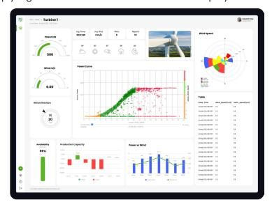
Our customers do not need to undertake costly software or service upgrades with their existing Scada systems, since Vis connects directly to the customer's Scada OPC data outputs and then displays the data locally and remotely, through existing communications systems.
